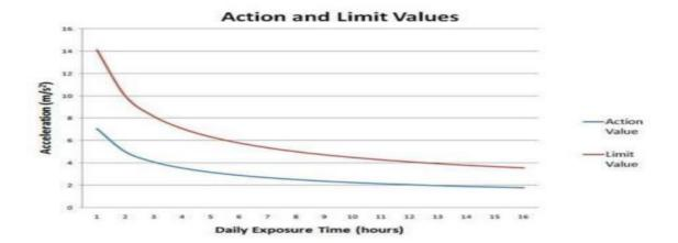
(For multi tool use we convert the ms2 value into Exposure points per Hour)
